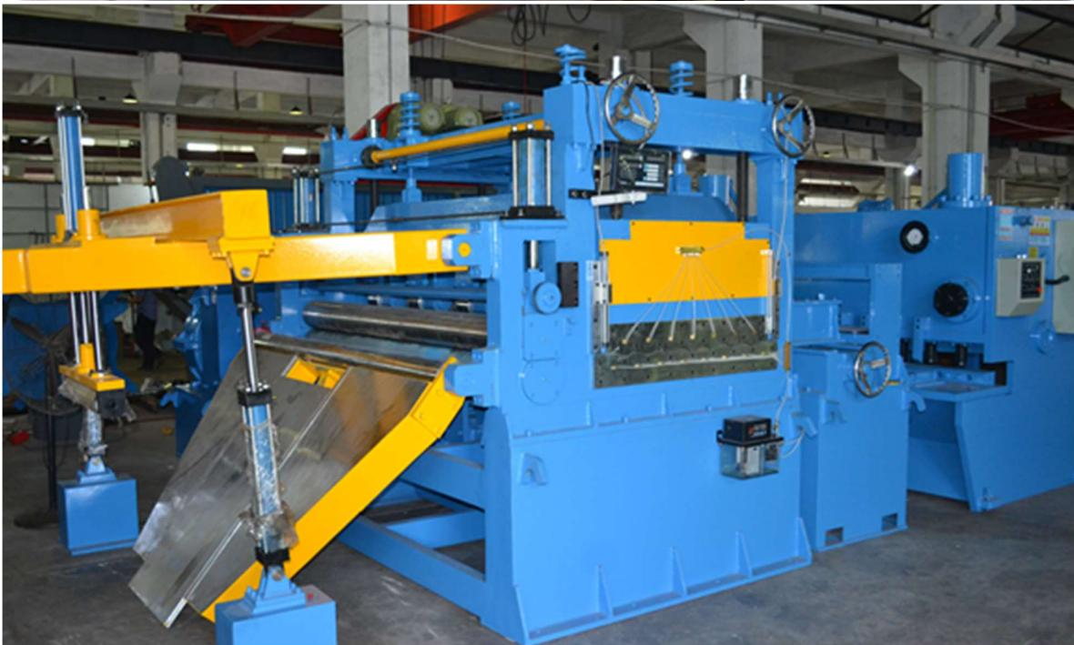
Cut to length line is a primary requirement in any service centre. We provide complete range of cut to length lines for all types of applications. We can provide from lines for thickness range from 0.1mm to 25mm, width up to 2500mm and speed from 20 to 120 meters per minute. We have specialised lines for Steel Mills, Service Centres, Auto Component manufacturers and various other applications.
