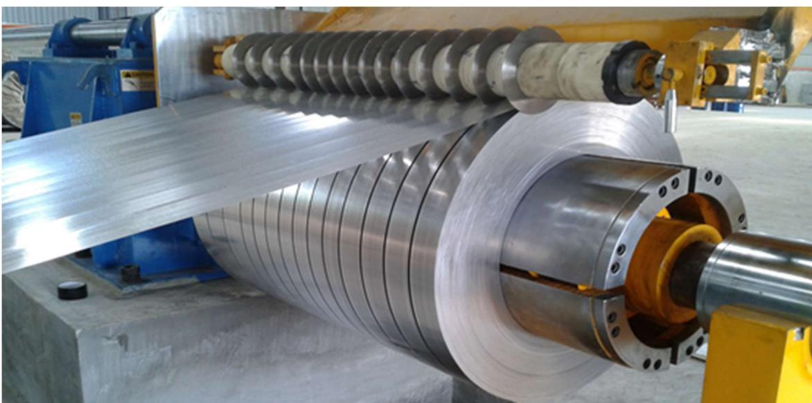
Slitting Lines are essential for Service centres and manufactures of Pipes, Angles, Channels, Purlins and Profiles. We can provide specialised slitting lines for all applications for low carbon steel, high carbon and stainless steel, aluminium coils and plates. We offer slitting lines up to 10mm thickness and width up to 2000mm and speed up to 180 meters per minute.
